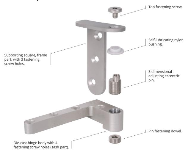
The eccentric pin allows the adjustment on 3 dimensions when door is installed.
