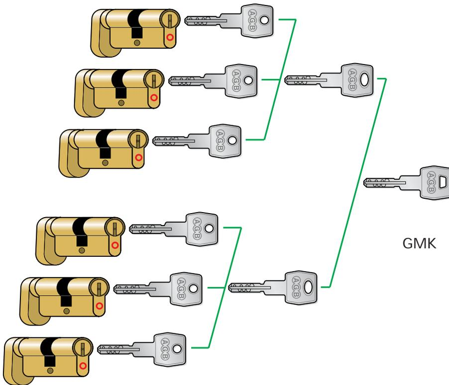
This is a master key system featuring multiple hierarchical levels where the cylinders are separated into several groups. Each cylinder is unlocked by its own key which cannot unlock any other cylinder of the system. Each homogeneous group of cylinders can also be unlocked by the group master key. All the cylinders of the system can be unlocked by the GMK general master key as well. This system can be utilized, for instance, in large hotels or in medium-large residential and public buildings.
